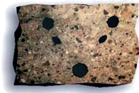
Cross-sectional view of a Pantex Lattice Girder integrated in shotcrete as performed on-site
