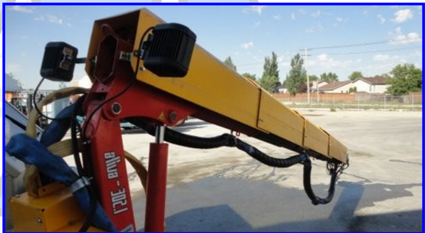
Figure 11 Aliva 302 boom and Work Lights
