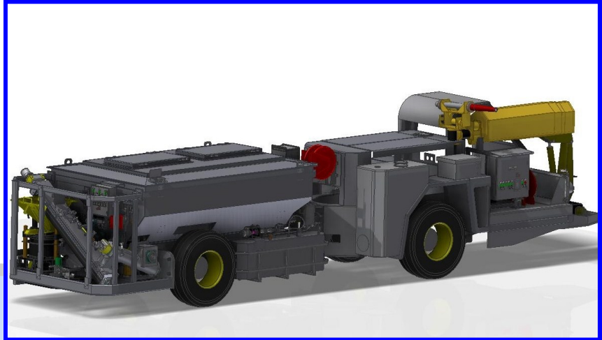
Figure 1 Aliva 302 Spray Boom (front) and Aliva 257 Wet/Dry Shotcrete Machine (rear) integrally assembled on Getman 64 Carrier.
