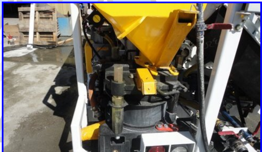
Figure 8 Aliva 257 Shotcrete Machine.
