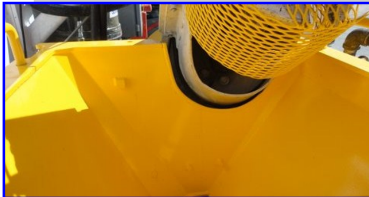
Figure 9 Mixing Auger & Aliva 257 Hopper
