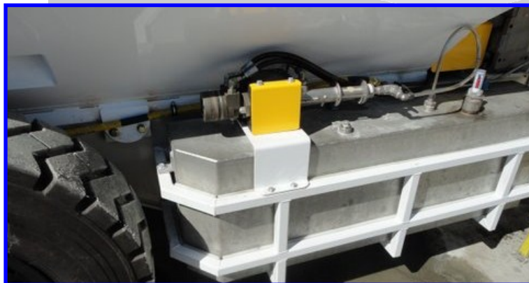
Figure 3 Liquid Accelerator Storage & Pump
