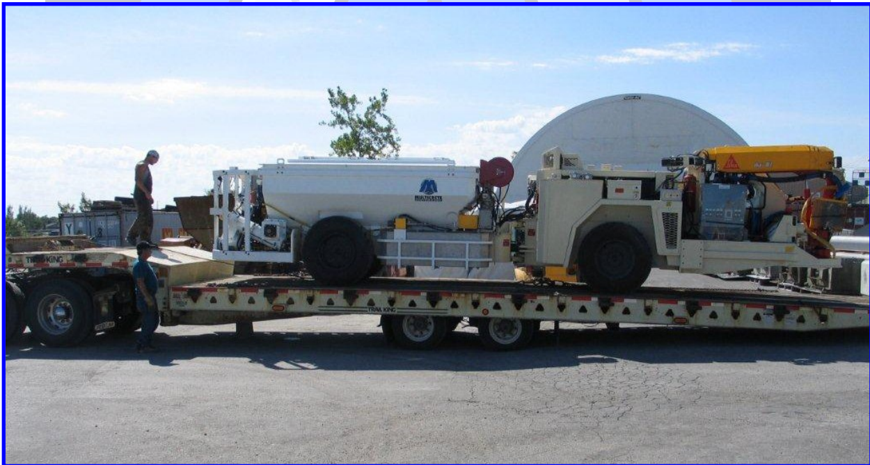
Figure 14 Multicrete Hybrid Wet ® Shotcrete Carrier-Ready to Ship
