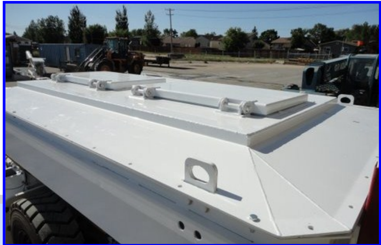
Figure 10 7 cu.yd Storage Hopper for Dry Pre-Mixed Product
