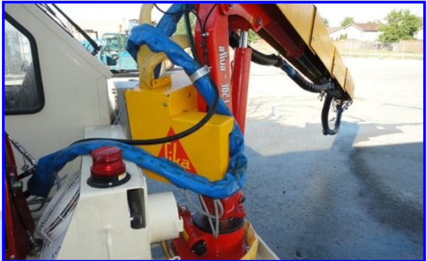
Figure 4 Aliva 302 Spray Boom with 240/360 degree Nozzle Rotation
