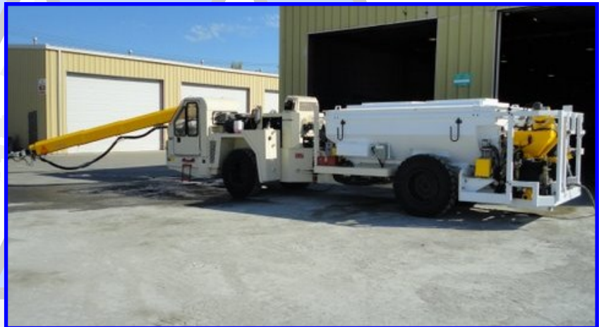
Figure 2 Aliva 302 Spray Arm extended
