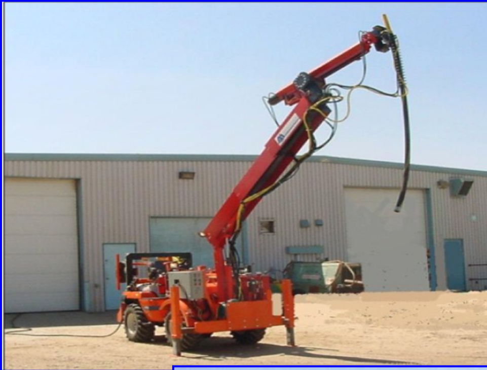
Figure 1 Fully extended Multicrete Auto Parallel Travel System demonstrating Vertical reach.
