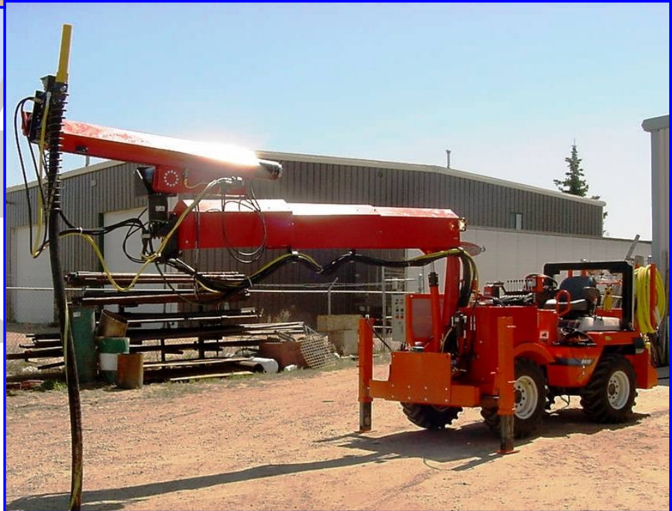
Figure 2 Fully extended Multicrete Auto Parallel Travel System demonstrating Horizontal reach.
