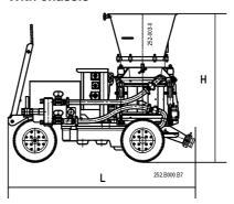
Length L with rotor 10 L 1770 mm with rotor 16L 1720 mm Width 800 mm Height H 1310 mm with rotor 10 L 1410 mm with rotor 16 L Weight approx. 760 kg Content of hopper 85 liters
