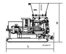
Length L with rotor 10 L 1640 mm with rotor 16 L 1590 mm Width 800 mm Height H 1260 mm with rotor 10 L 1360 mm with rotor 16 L Weight approx. 800 kg Content of hopper 85 liters
