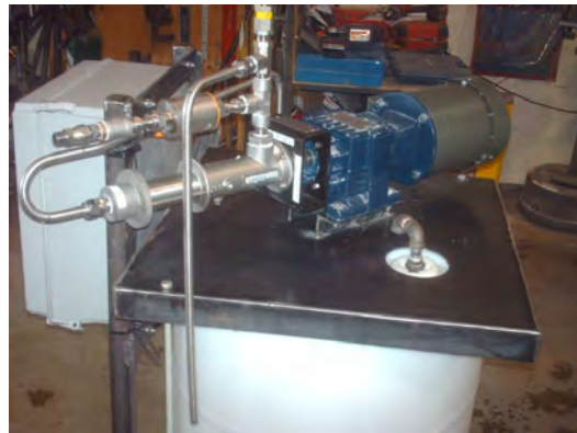
Peristaltic Hose Pump Guarantees smooth steady flow
