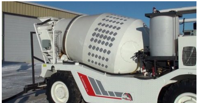
Figure 2: Mixing drum and liquid accelerator storage.
