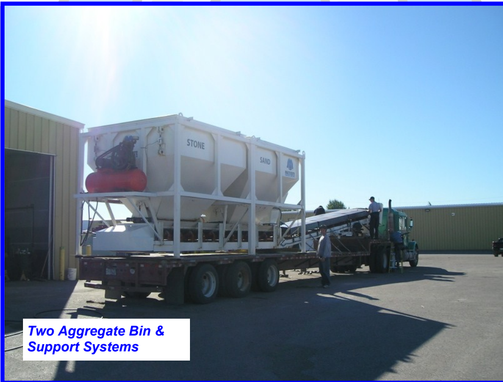
Conveyor & Weigh Hoppers
